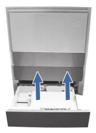
9. Make sure that the tray width and length guides are set to the correct paper size for the paper being installed into the tray and that the tray is not over filled above the fill mark (line below 3 triangles on rear guide).
