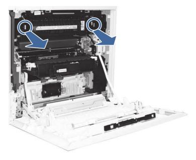
b. Remove any paper jammed in the fuser exit area.
