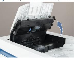
b. Release the blue locking arm to drop the assembly down. Slide the pickup and feed roller assembly to the left, and then pull it away from the document feeder to remove it.
