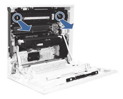
b. Remove any paper from the exit of the fuser.
