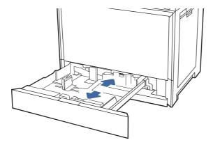
3. Adjust the paper-length guide by pushing in at the bottom of the blue adjustment latch while sliding the guide to the size of the paper being used.
