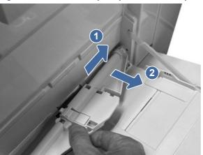
c. Grasp the left- and right-side of the separation roller assembly, and then lift the assembly up.
