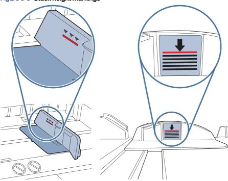
Figure 9-7 Tab for the paper stack
