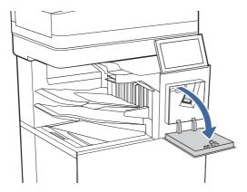
2. Pull down the colored handle on the staple carriage, and then pull the staple carriage straight out.
