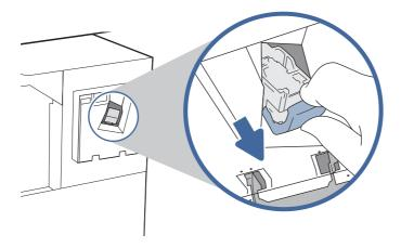
3. Remove the staple cartridge from the sled and replace it with the new staple cartridge.
