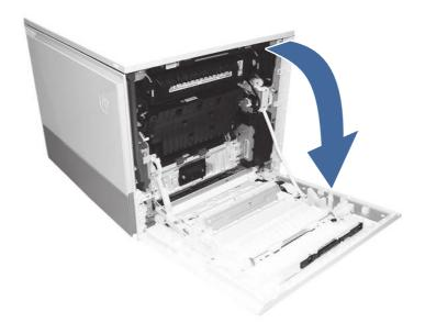
4. Remove the fuser and remove any jammed paper found.
