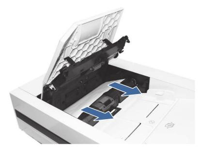
4. Lift the document feeder and check the lower side of the feed path.
