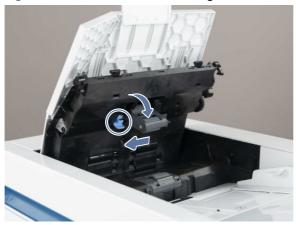
c. Lift the roller cover up and then slide the roller toward the front of the printer to remove it.
