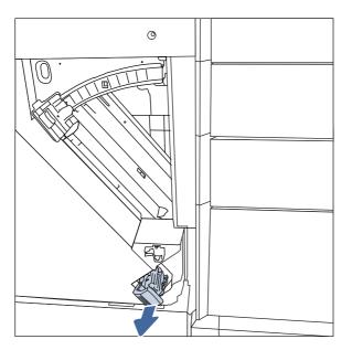
3. Remove the staple cartridge from the sled and replace it with the new staple cartridge.
