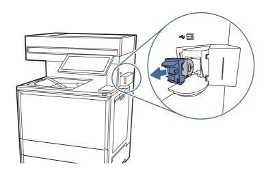
3. Insert the new staple carriage into the stapler.
