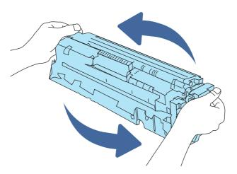
5. Align the toner cartridge with its slot and insert it into the printer.
