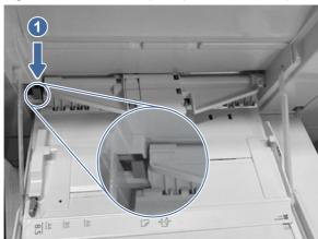
b. Push the pickup roller assembly to the right and then away from the printer.
