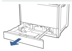
2. Before loading paper, adjust the paper-width guides by holding down the blue lock/unlock toggle switch on the rear paper-width guide, pinching the blue adjustment latch on the front paper-width guide, and then sliding the guides to the fully open position.
