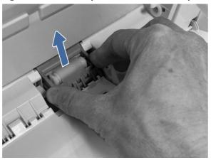
d. Pull the separation roller assembly straight out to remove it.
