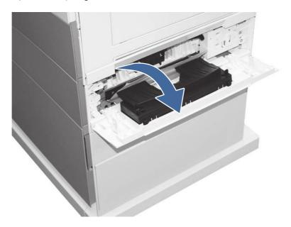
b. Locate and remove the Tray 3 separation roller.
